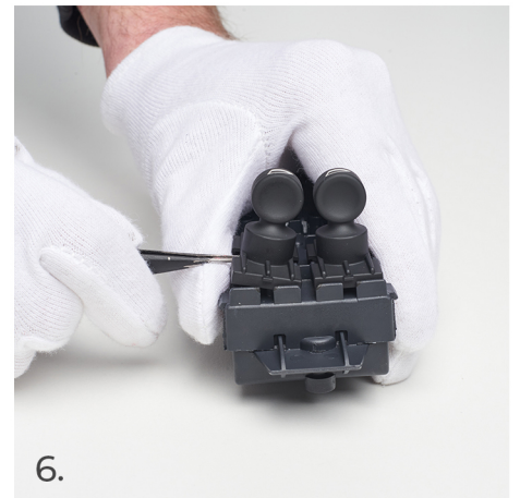
6. Stop in this position when the switch is free on one side.
