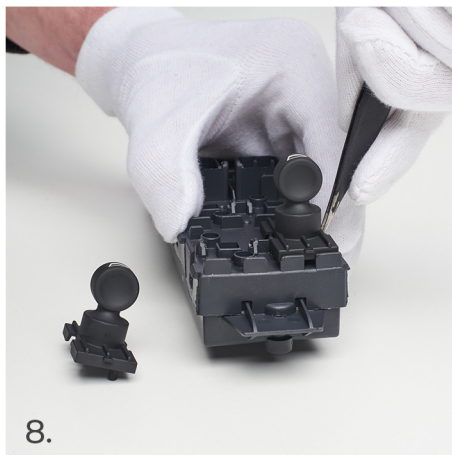
8. Always start from the outside of the switch. Start from the top and place the tweezers in the area shown in the previous image.
