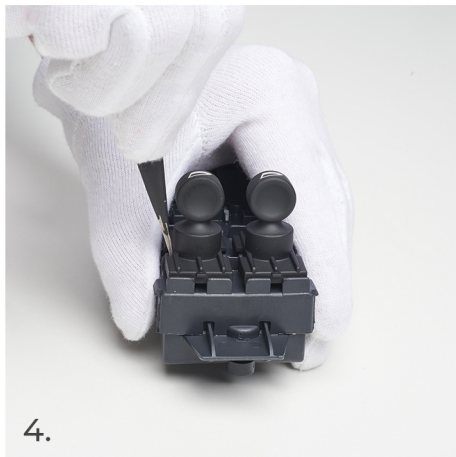
4. Gently pry the switch with the top of the tweezers.
