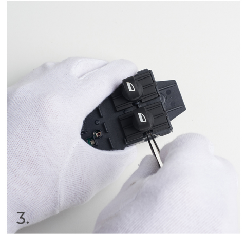
3. Always start from the outside of the switch. Start from the top and place the tweezers in the area shown in the previous image.
