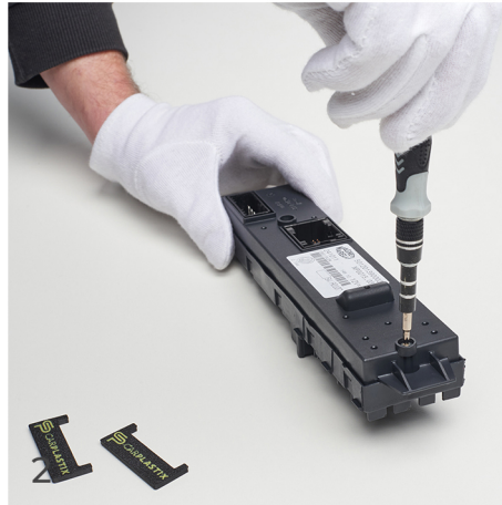
Unscrew the first screw at the bottom of the assembly.
