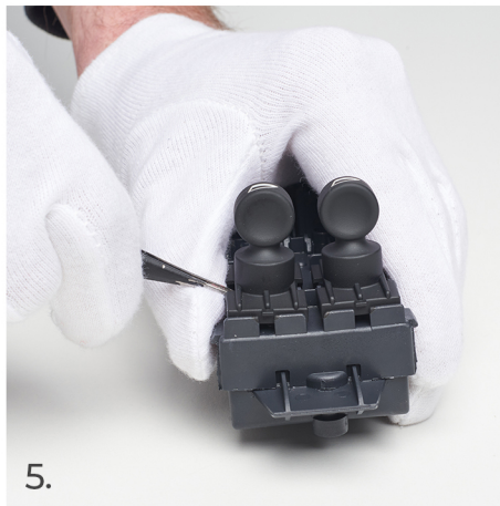
5. Gently pry the switch with the top of the tweezers.
