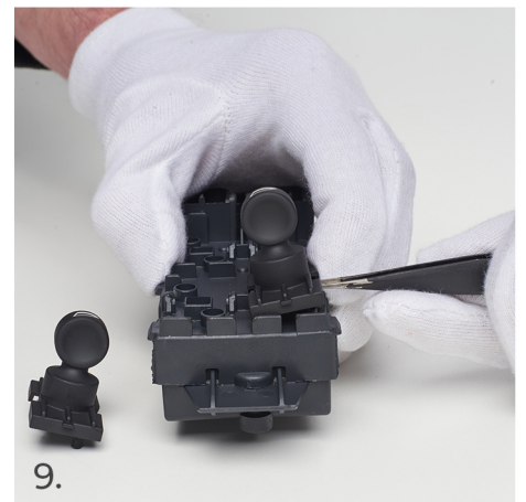
9. Gently pry the switch with the top of the tweezers. Proceed in the same way as with the previous switch.
