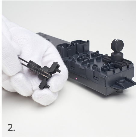
2. This is where you need to place the top of tweezers to prevent switch damage.
